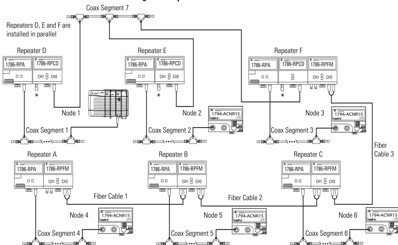
Repeaters A, B, and C are installed in series and connected to the repeaters in parallel on segment 7 via Repeater F
