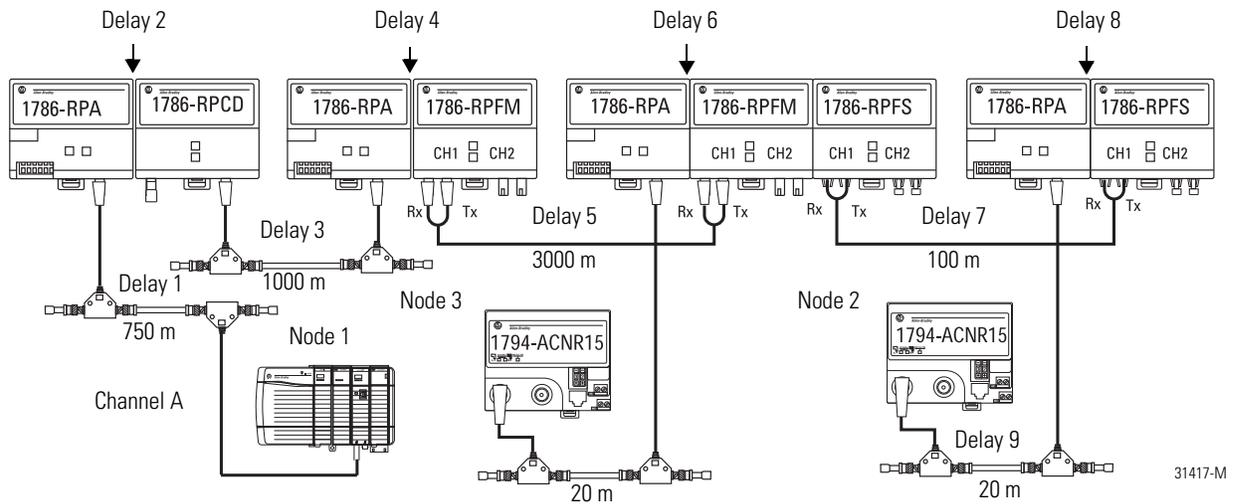
The example has the following maximum delay path from node 1 to node 2, end to end.
