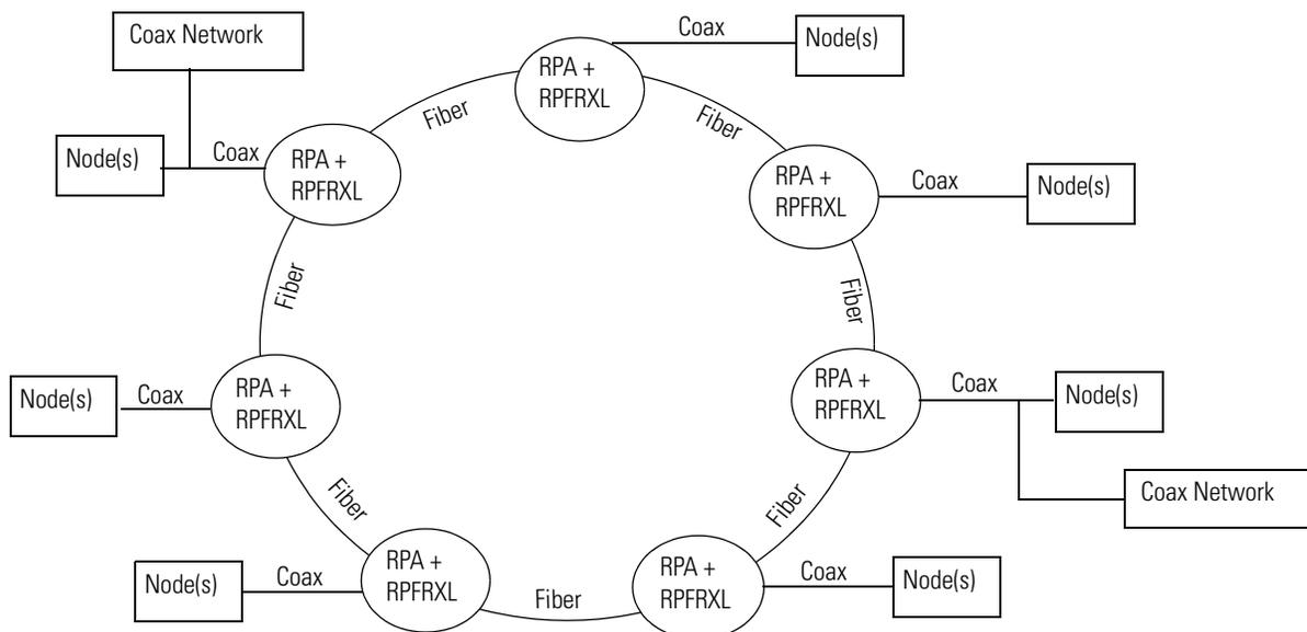
If a ring is broken, the configuration then becomes a linear bus and the number of repeaters in SERIES depends on where the ring is broken. You will have as many repeaters as in the original ring.
