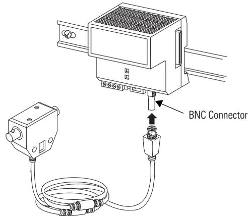
6. Terminate any unused coax ports by connecting a  $75\ \Omega$  terminator to the unused BNC connector.
