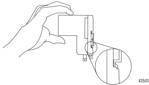
**TIP** Use a screwdriver to move the locking tab downward, if the module is not secured.
