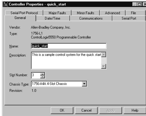
3. Configure the controller by specifying the slot number of the controller and the chassis size.
